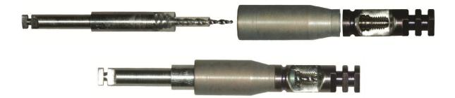
4. Modified drill prototype, guide and windowed analog both separate and assembled.
